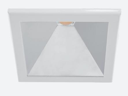
Recessed square LED luminaire. Body is made of steel and aluminium and it is available in all RAL colours. Light source - Philips, Osram or Tridonic LED module. Standard EVG ballast, DALI or Touch Dali version on request. Passive cooling, optional IP44 diffuser: Product is also available with special application LED modules: CrispWhite, Food WarmWhite, Food PremiumRed and many others - details on request.
